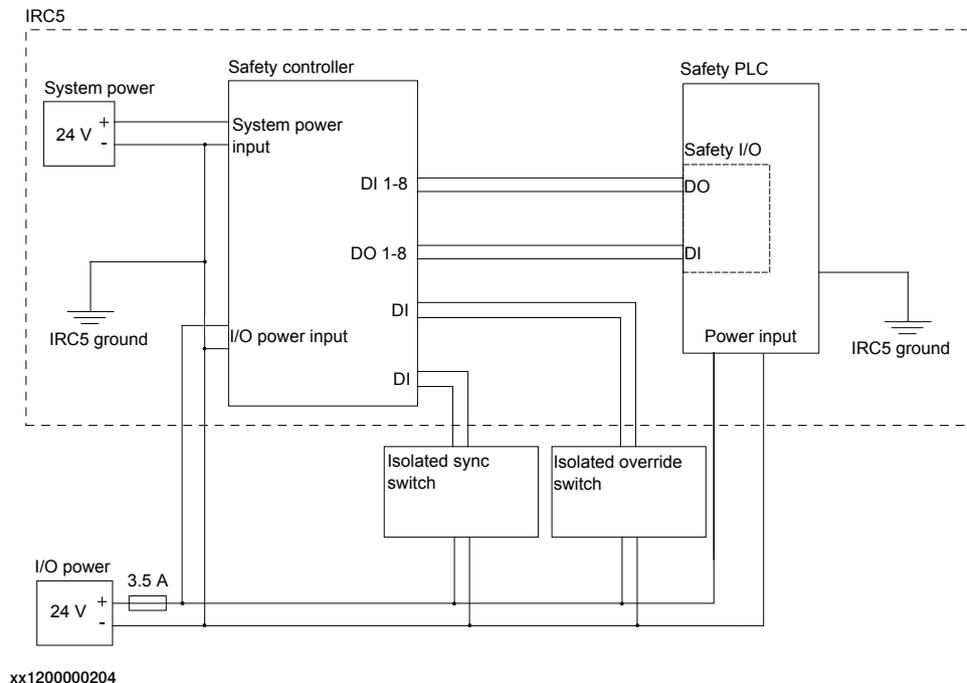
For a single cabinet IRC5 controller, the I/O power supply can be an internal power supply located in the IRC5 cabinet. For a dual cabinet IRC5 controller, an external power supply needs to be used.
